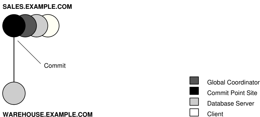
Figure 34-8 Determining the Commit Point Site
